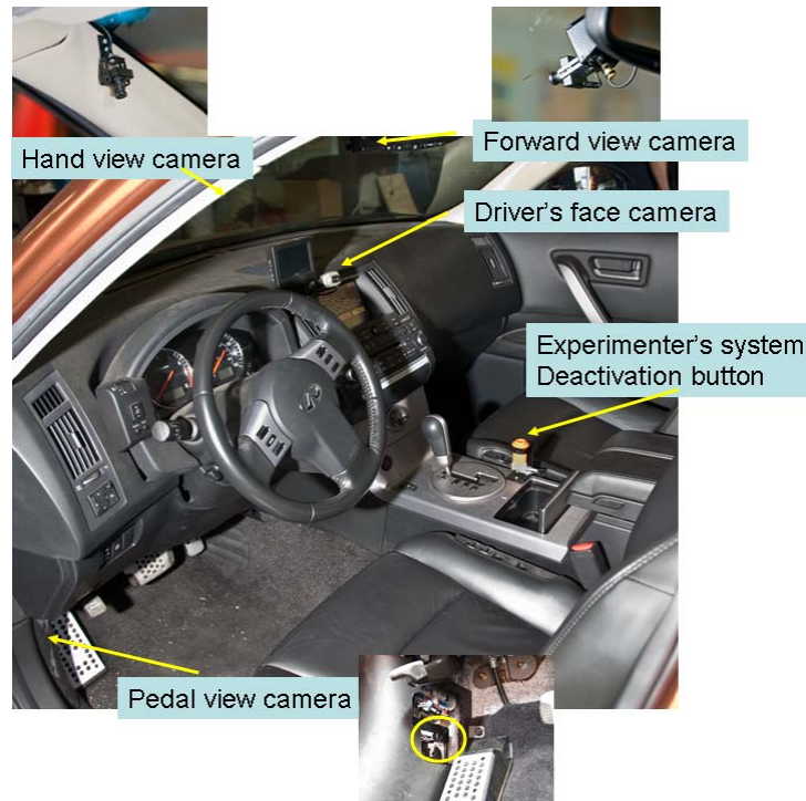
Figure 4.4: Vehicle Interior, Showing Locations of Video Cameras
