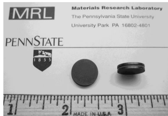
Figure 1.4. Magnetoelectric lamina composite using Terfenol-D and PZT disks. (Figure from [21])
