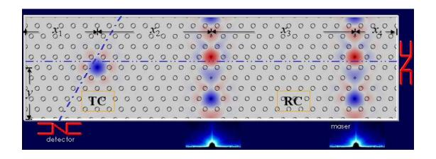
Fig. 1. Illustration of the proposed photonic crystal quantum circuit. This illustration is not to scale. guneyF1.eps.
