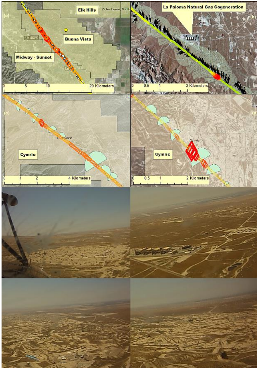
Figure 3. 14. Flight segment over oil and gas fields in western Kern County color coded by CH 4 concentrations. The spatial extent of the oil fields are shown as a semi-transparent overlay with the black arrows and half-dome footprints indicating incoming wind direction and representative fetch, respectively. The plots depict flight stretch over (a) Midway-Sunset and Buena Vista oil field; (b) La Paloma natural gas cogeneration plant; (c) and (d) Cymric oil field. The bottom four images are taken from the on-board GPS enabled high-definition video camera and shows the real time image capture of oil and gas operations and the natural gas co-generation facility.
