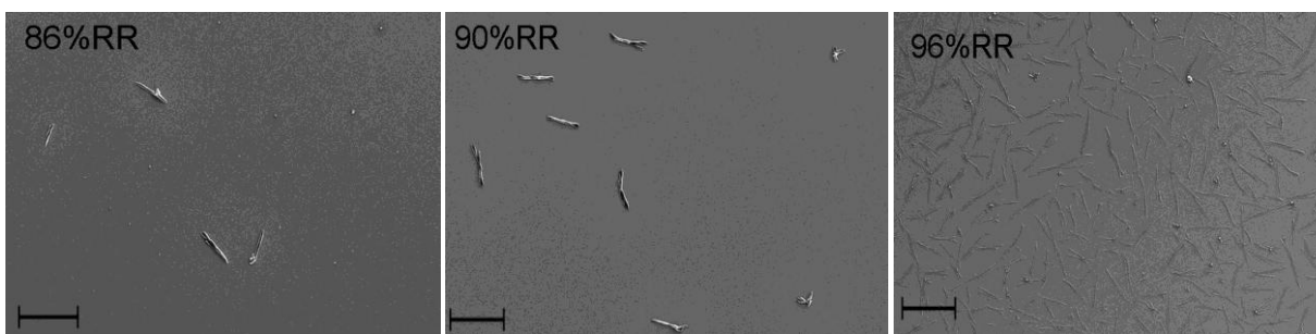
Figure 2.7. SEM images of P3HT: PCBM blend films at 55:45 weight ratio annealed at 150°C for 3 hrs. Scale bar = 100 \mu m.
