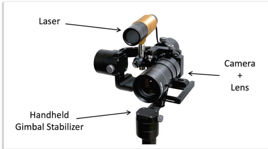
Figure 2.2: Motion Stabilized Laser Speckle Imaging (msLSI) Device. Fully-assembled device utilizing a gimbal stabilizer with the laser speckle imaging device.
