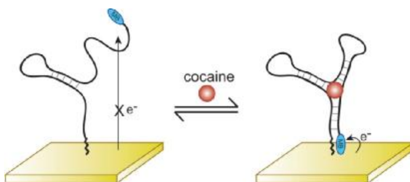
Figure 1-2. The cocaine E-AB sensor is comprised of an unfolded, electrode-bound sensing aptamer. Cocaine binding traps the aptamer in its folded state, forcing an attached redox reporter (here we have employed methylene blue -MB) into proximity with the electrode, leading to a large change in Faradaic current.
