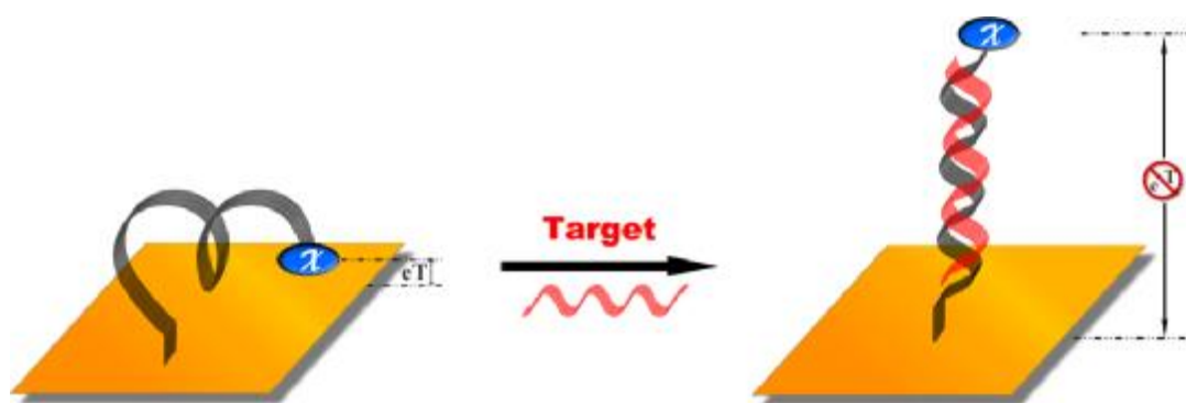
Figure 1-1. Signal generation in the electrochemical DNA (E-DNA) sensor occurs when hybridization with a target oligonucleotide reduces the efficiency with which the attached redox reporter (X) can approach the electrode and transfer electrons.
