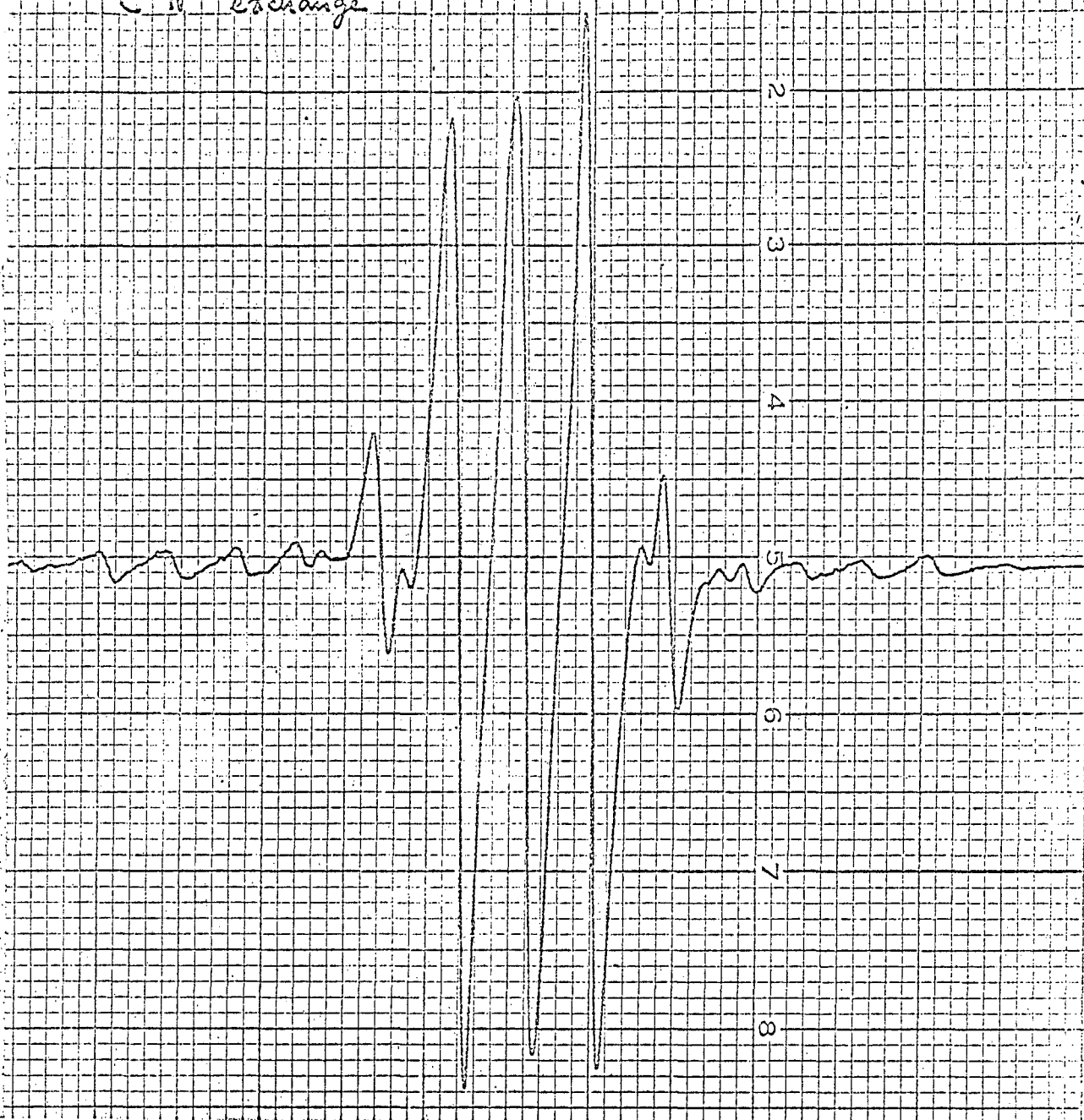
Figure 1. The center triplet is due to N^{14}O^+ , the single line on either side is due to partially exchanged C^{13}N^- and the weak lines are mainly Cr^{53} .
