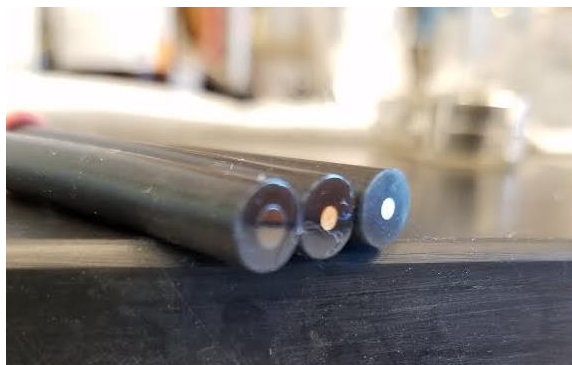
Figure 2.4 Photo of (left to right), 3.0 mm diameter glassy carbon, 1.6 mm gold and 1.6 mm platinum disc working electrodes, which are manufactured in a solvent resistant plastic body (BASi).
