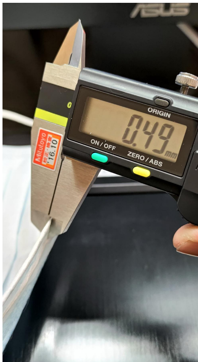
Figure 1 Measurement of the physical thickness of a single piece of medical mask using a commercialized caliper.
