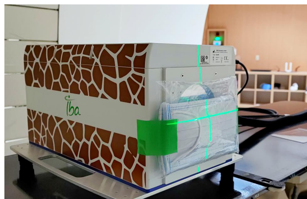
Figure 2 Measurement of the water equivalent thickness of medical masks in 10-piece packs.
