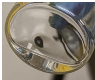
Figure 5.11. No gelling of sample dissolved in \text{D}_2\text{O} , after washing with ethyl acetate.
