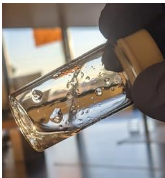
Figure 5.7. Gelled solution from spontaneous polymerization of functionalized urea monomer product in \text{D}_2\text{O} .
