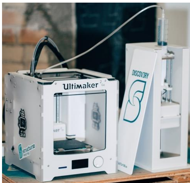
Figure 2.3. Original Discov3ry Complete Paste Extruder. The enclosure to the right of the Ultimaker 2+ houses the syringe pump. [Adapted in part with permission from Discov3ry Complete. Structur3D Printing Home Page. https://www.structur3d.io/ (accessed 2018-01-01) Copyright 2016, Structur3d Printing.]
