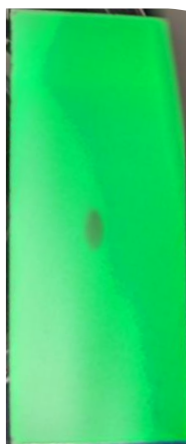
Figure 5.3. TLC plate with spot corresponding to pure MAMPSA monomer.
