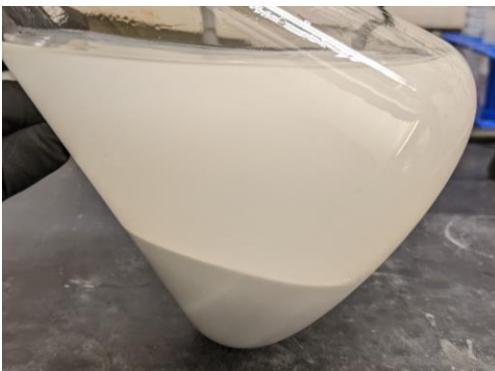
Figure 5.2. Crude MAMPSA product dissolved in DCM with NaI precipitate on bottom.
