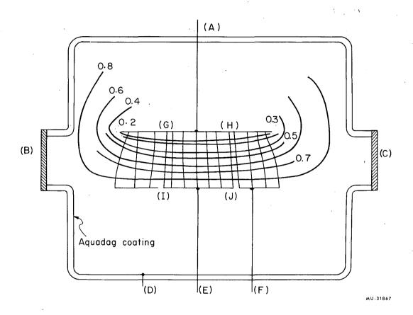
Fig. 3. Side view of equipotential surfaces and flux lines in reaction cell: (A) high-voltage terminal; (B) LiF window to lamp; (C) LiF window to lamp-intensity monitor; (D) Aquadag-coating terminal; (E) collecting-plate terminal; (F) Guard-ring terminal; (GHIJ) cross section of actual collection volume.
