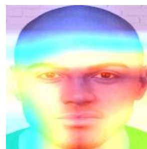
Figure 3: Sample output from Grad-CAM. Redder colors are more important for the decision, bluer colors are less important.
