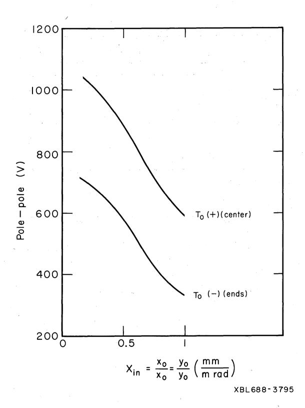
Fig. 3 Quadrupole voltages for triplet  $T_0$  as a function of  $X_{in}$ , for 10 keV proton beam.
