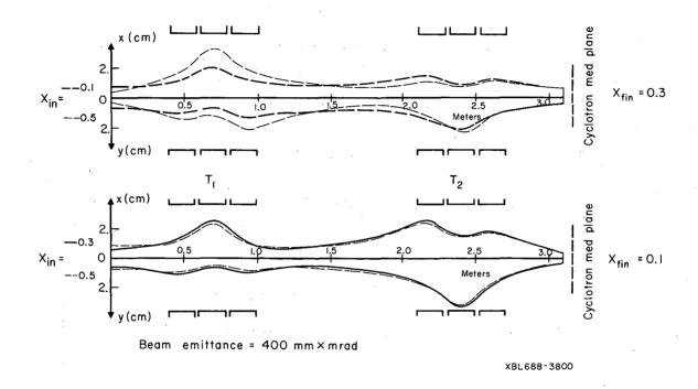
Fig. 7 Typical beam envelopes through triplets  $T_1$  and  $T_2$ , for several  $X_{in}$  and  $X_{fin}$ , and waist position at 5 from the cyclotron median plane.
