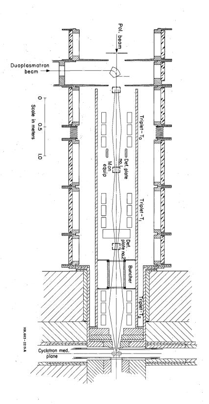
Fig. 1 Layout of the axial injection line. Only schematic beam envelope is shown.
