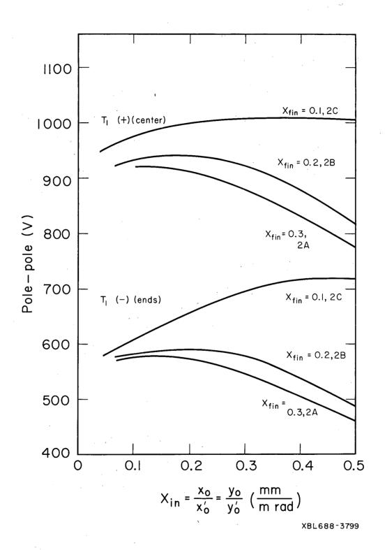
Fig. 6a Quadrupole voltages for triplet  $T_1$  as a function of  $X_{\rm in}$ , for  $X_{\rm fin}=0.3$  (2A), 0.2 (2B), 0.1 (2C), and final waist position at 15 cm from the cyclotron median plane (Solution 2, 10 keV protons).
