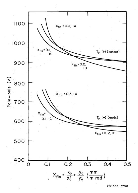
Quadrupole voltages for triplet  $T_2$  as a function of  $X_{in}$ , for  $X_{fin} = 0.3$  (1A), 0.2 (1B), 0.1 (1C) and final waist position at 5 cm from the cyclotron median plane (Solution 1, 10 keV protons).
