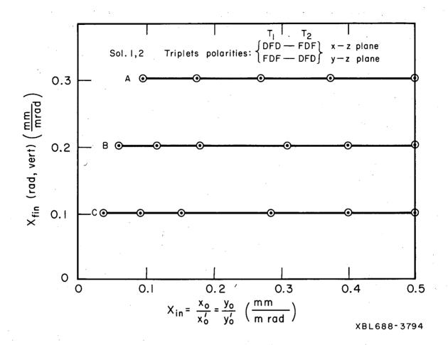
Fig. 4 Diagram  $X_{fin} = X_{fin} (X_{in})$  for the available matching solutions. Circles indicate computed points.
