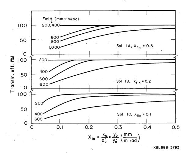
Fig. 8 Transmission efficiencies for beam emittances of 200, 400, 600, 800 and 1000 mm mrad over a range of  $X_{\rm in}$  and  $X_{\rm fin}$  values. Final waist position at 5 cm from the cyclotron median plane (Solution 1).
