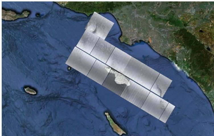
Figure 4.3: SAR georeferenced map of mosaiced images from 04.15.2011 provided by the JPL operated Gulfstream jet. The *.kmz extension files are compatible with Google earth maps, or other map programs.
