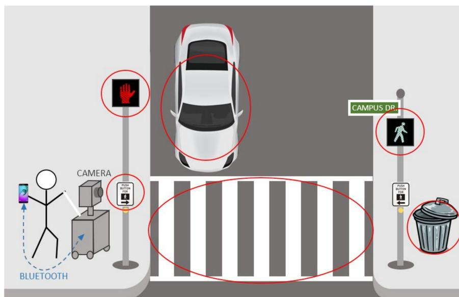
Objects circled red are detected by RoboEye. Some objects are detected and avoided, others send a signal to wait before crossing.
