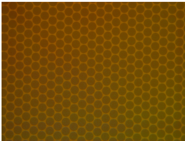
Figure D.36. Hexagonal matrix of 10um holes, 1um separation.
