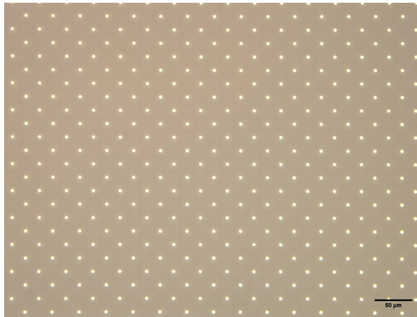
Figure D.23. Simple Cubic Matrix of 5um islands, 20um separation.
