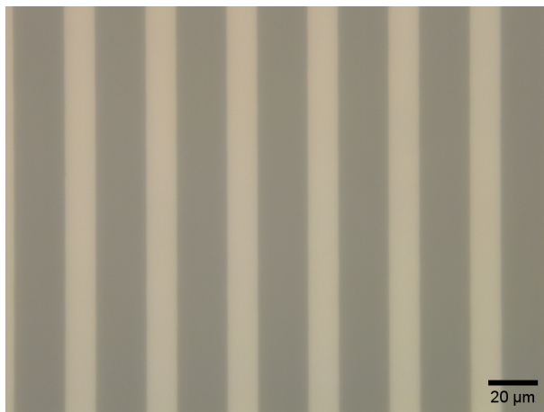
Figure D.25. Optical Grating 20um Slit, 12.5um spacing.
