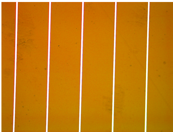
Figure D.31. Grating (nanowires): 200um slit, 10um spacing.
