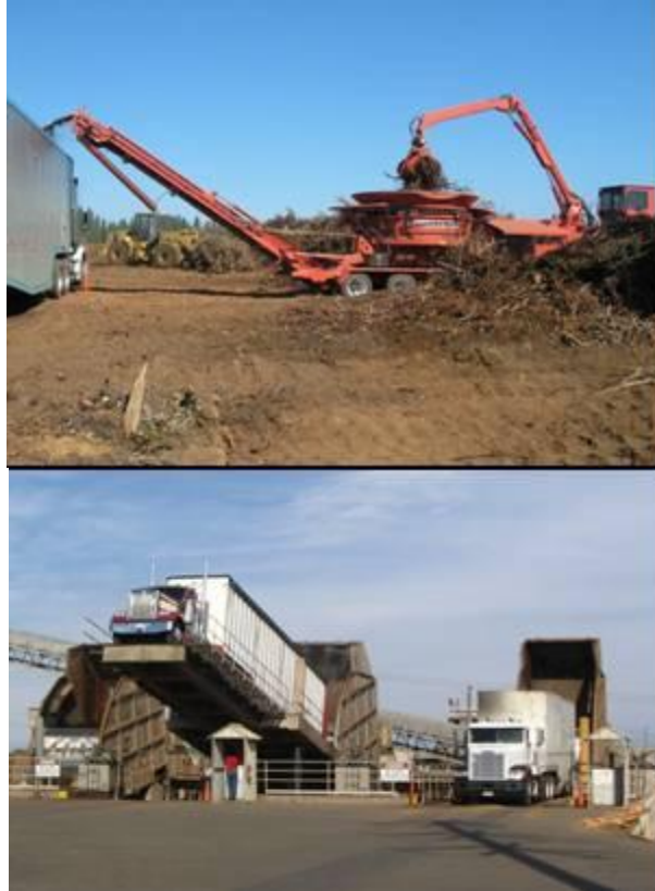
Figure 4. Grinding and removal of brush from Red River Forests Partnership site to Wheelabrator Shasta biopower plant
