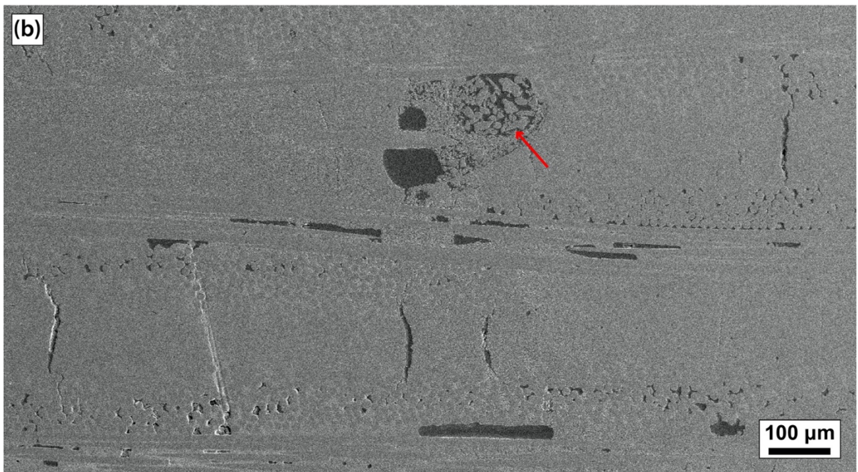
Figure 5.10: SEM cross-section of the N = 4 , fully impregnated, y_p = 6.2\% alumina precursor sample, with arrows highlighting large voids filled with precursor derived alumina (a) near the surface and (b) deep in the middle of the composite.
