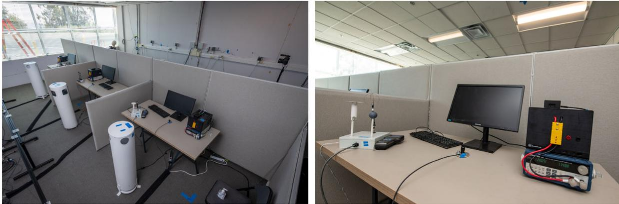
**Fig. 5.** Photograph of cubicle-partitioned workstation layout in test cell (left), with programmable plug loads visible on desks. White cylinders are occupant thermal generators at each workstation. A close-up view of a workstation is visible in the photograph on the right, showing programmable load on the desktop as well as illuminance sensor and thermal comfort station measuring dry bulb temperature, mean radiant temperature, relative humidity, and airflow velocity.
