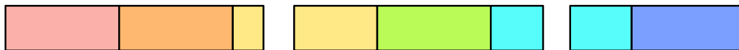
(b) Reader threads read data into fixed size memory regions based on the properties of the storage devices. This can fragment records across memory regions.
