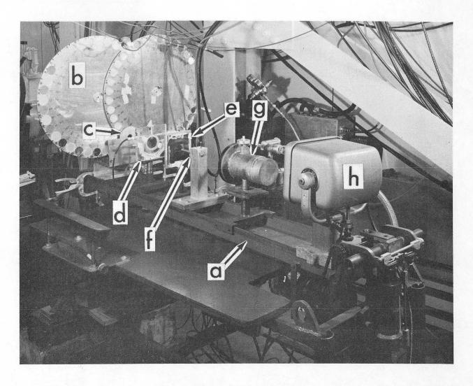
Fig. 3. Adjustable irradiation table: (a) alignment rail, (b) absorber wheel, (c) collimator, (d) ionization chamber, (e) cross hairs, (f) pointer, (g) Faraday cup, (h) x ray source.
