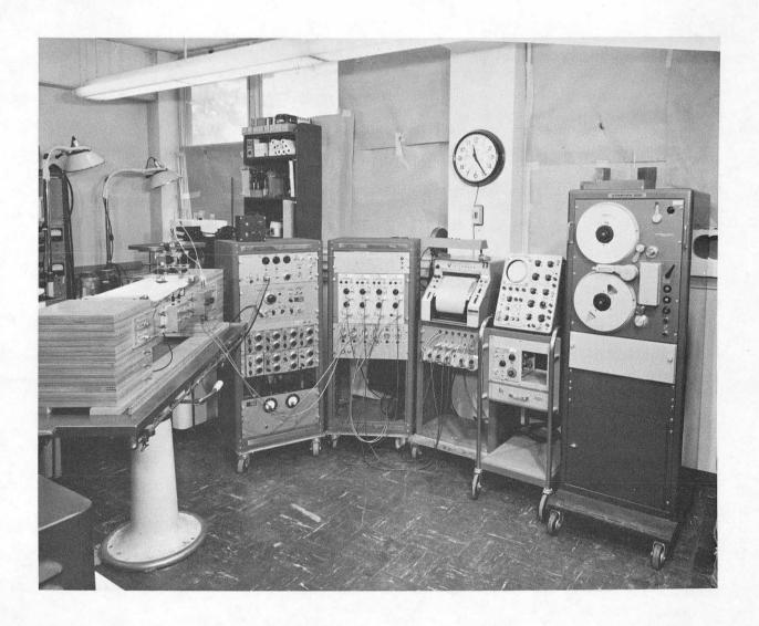
Fig. 9. Stimulating and recording system, and physiological preparation equipment.
