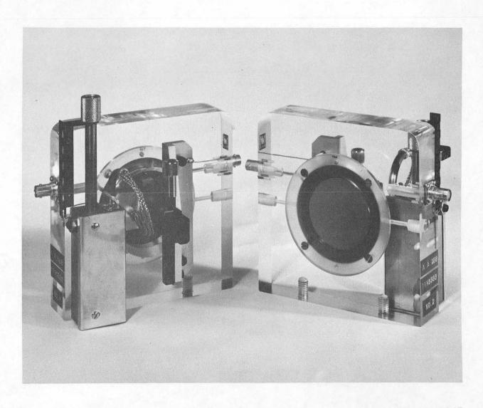
Fig. 4. Variable gap - variable collector ionization chamber.
