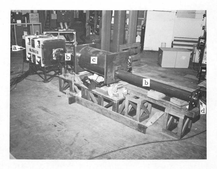
Fig. 12. Beam transport system: (a) quadrupole, (b) beam tube, (c) beam plug, (d) vacuum window.
