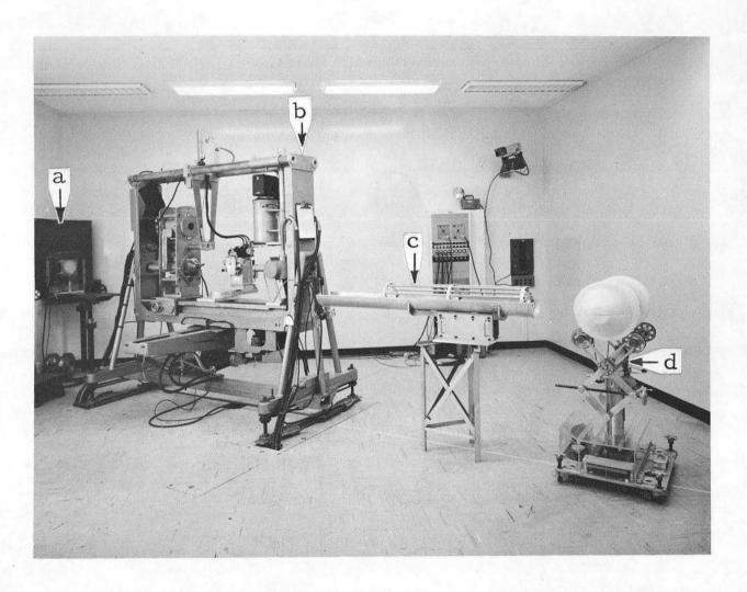
Fig. 14. Interior view of the medical cave: (a) scattering-target exit, (b) human positioner, (c) scattering-target loading device, (d) animal-rotator.
