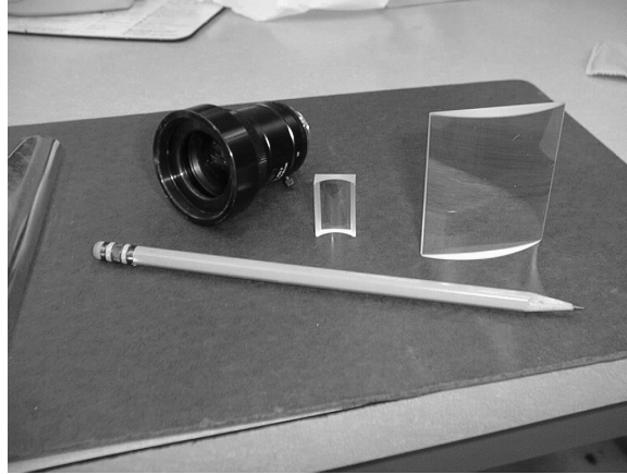
Figure 2.5: Imaging Lens and Cylindrical lenses
