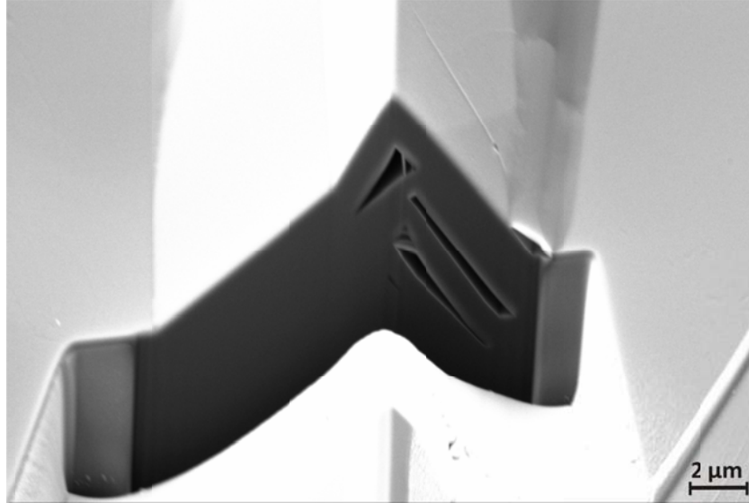
Fig. 54. Cross section of a wrinkle by Focused Ion Beam cutting
