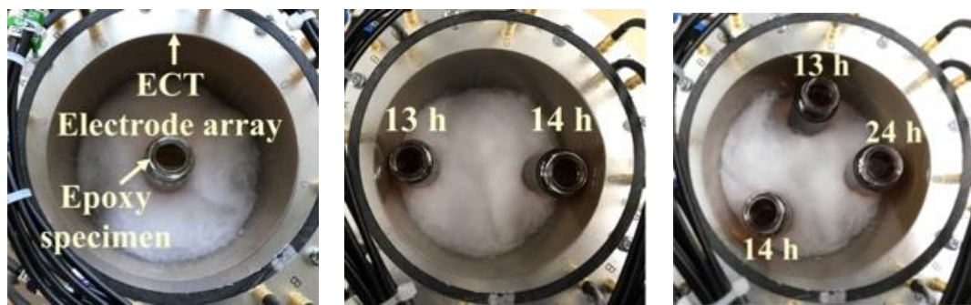
Figure 3.3. (a) An epoxy specimen is placed in the electrode array for ECT interrogation and data acquisition. (b) Two epoxy specimens subjected to 13 h and 14 h of curing were also simultaneously interrogated, (c) followed by testing three specimens cured for 13, 14, and 24 h.
