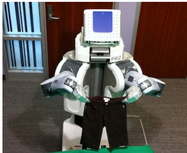
Fig. 2: The PR2 holding up the pair of pants after starting with the configuration shown in Figure 1.
