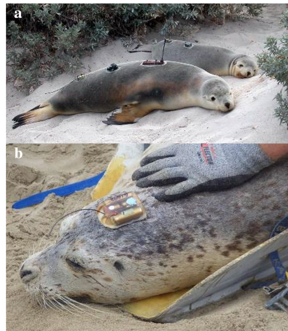
Fig. 3 Examples of optimal EDT configuration and attachments. a Australian sea lion adult female and 6-month-old pup at Kangaroo Island, South Australia, part of a research project investigating the ontogeny of diving and movement behavior and physiology [32]. The adult female is instrumented with (from head to tail) an Argos satellite transmitter (Telonics Inc., Mesa, AZ, USA), a Mk-6 depth and swim velocity data recorder (Wildlife Computers, Redmond, WA), and a VHF beacon (Lotek/Sirtrack, St. John's, Canada). The pup is carrying a Mk-5 depth data recorder (Wildlife Computers) and a VHF beacon (Lotek/Sirtrack). 6-month-old pups were not instrumented with Argos transmitters because earlier observations indicated that they did not leave the colony until they were older, making the additional instrument unnecessary (Recommendations # 1, 3, and 4). The instruments were attached to the animals using a 2-part quick-setting epoxy, with a layer of neoprene and mesh between the tag and pelage to allow for easy removal during recapture (Recommendation # 9). Tags were attached in line along the dorsal surface to minimize disruption of laminar flow around the animal (Recommendation # 8). Photo © DP Costa, 2002, South Australian Department for Environment and Heritage permit #G24475-2. b Attachment of a SPOT Argos transmitter (Wildlife Computers, 72 × 54 × 24 mm, 119 g) to the head of an adult Pacific harbor seal in Oregon. The base of the tag was built up into a convex shape to conform to the curvature of the skull, and is then directly glued to the pelage surface with Loctite™ Type 422 ethyl-cyanoacrylate adhesive (Henkel Corp., Düsseldorf, Germany). No mesh is used to minimize the contact area to the tag footprint (Recommendation #9 and 10). This adhesive sets within 10–30 s, and may generate some heat in the process. An alternative that produces less reaction heat for work in warmer climate can be found in Loctite™ Type 4861 ethyl/butyl cyanoacrylate that cures within 60s without generating much heat in the process. Type 4861 remains flexible on curing. However, achieving proper curing can be challenging, and may be facilitated through the use of accelerants (water or acetone mist). This deployment was part of an investigation into the spatial behavior of harbor seals, their use of marine reserves, and environmental drivers of their movement [110]. The lightly sedated animal is being immobilized on a V-shaped restraint board during the attachment (Recommendation # 6). Photo © SM Steingass, 2015, NMFS #16691
