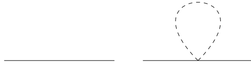
Figure 1.3: The two Feynman diagrams that contribute to the \frac{1}{2}\mu^2(\Lambda)\phi^2 in the effective Lagrangian up to order \lambda^2 . The dashed lines indicate the large |p| fields that are integrated out while the solid lines are the low |p| that remain in the effective Lagrangian.
