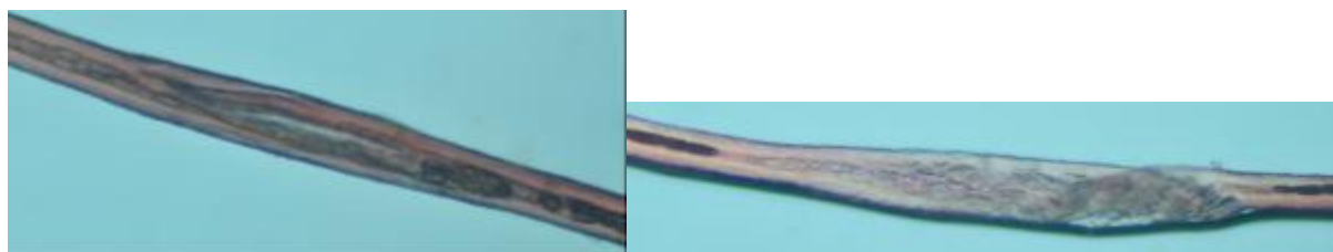
Figure 13. Secondary electron micrographs of fibers from sample T-130A, displaying crease and folds in the fiber, perhaps do to exposure to an alkaline environment during burial.
