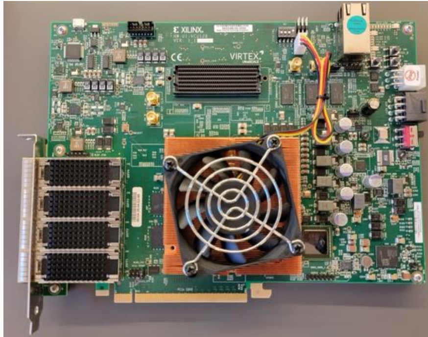
Figure B.1: Xilinx Virtex Ultrascale+ HBM (VCU-128) FPGA Board. Board includes Xilinx VU37P FPGA with 2 \times 32Gb 4H HBMs.
