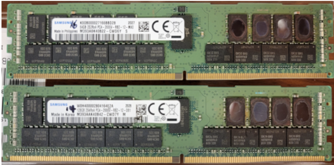
Figure B.3: Delidded 3D-Stacked (3DS) DRAM Memory. 288-pin DDR4 modules were utilized for testing. A 64GB, 2-layer stacked DIMM ( top ) and a 128GB, 4-layer stacked DIMM ( bottom ) were used for testing. Devices D21-D24 were delidded—device #'s [Sam17a] & [Sam17b]. Devices D25-D28, directly below the delidded devices, were also utilized for testing at the NASA Space Radiation Laboratory (NSRL).
