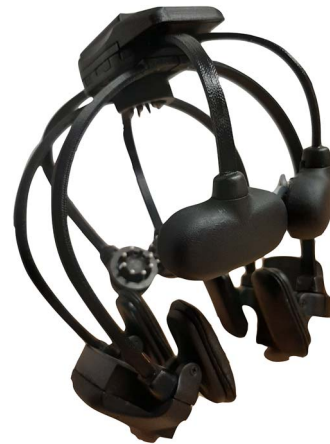
Figure 2. EEG equipment. Mobile, dry EEG headsets designed by Cognionics and employed to collect neural data.
