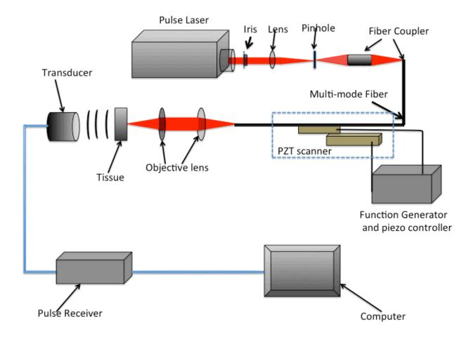
Figure 14 Schematic of PZT-Photoacoustic Microscopic System
