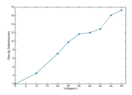
Figure 8 Fiber –tip deflection versus voltage applied on PZT of 1-D PZT scanner
