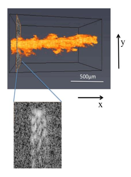
Figure 23 The 3-D PAM image of the mechanical pencil lead
