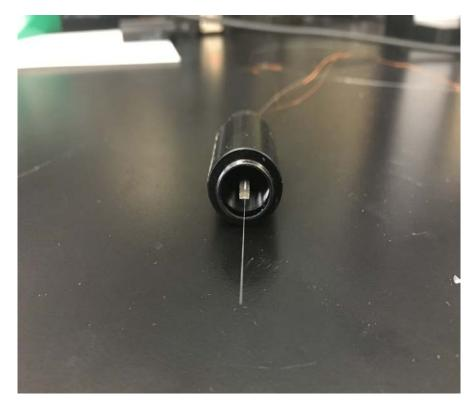
Figure 5 1-D PZT scanner placed in a half-inch tube
