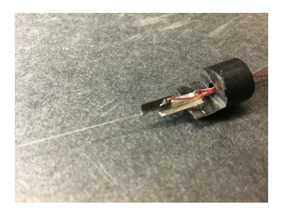
Figure 13 The 2-D PZT scanner
