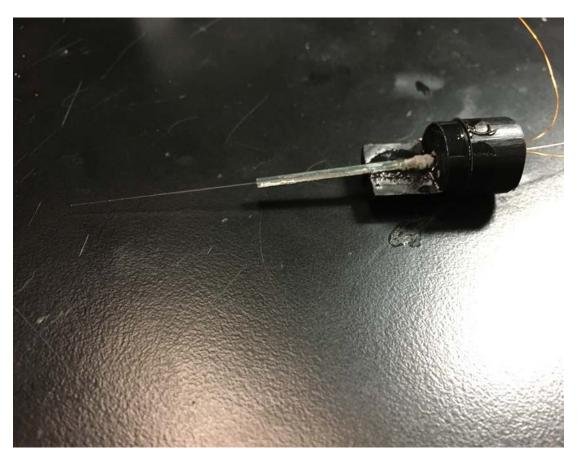
Figure 4 One-dimensional PZT Scanner
