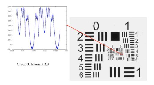
Figure 17 Scanning Group 3, Element 2 and 3 of resolution target
