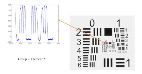
Figure 16 Scanning Group2, Element 2 of resolution target
