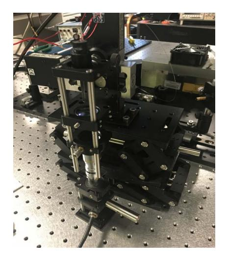
Figure 22 2-D PZT scanner based imaging system
