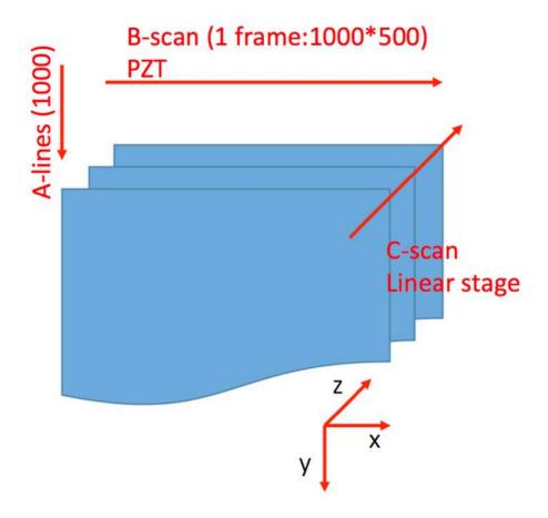
Figure 20 2-D scanning mechanism for 1-D PZT scanner
