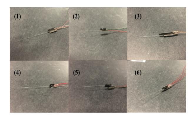
Figure 9 The 2-D PZT Scanners
