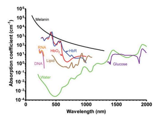
**Figure 1** Absorption spectra versus wavelength of several endogenous contrast agents on biological tissue\*
