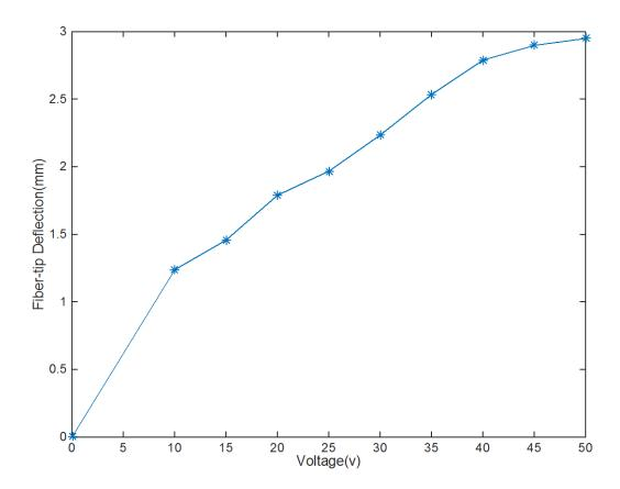
Figure 12 Fiber-tip deflection versus voltage of 2-D PZT scanner
