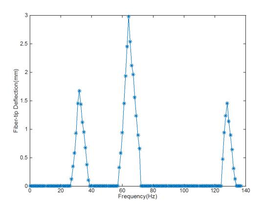
Figure 11 Fiber-tip deflection versus frequency of 2-D PZT scanner
