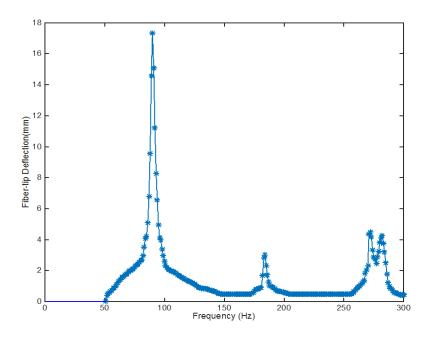
Figure 7 Fiber-tip deflection versus frequency of 1-D PZT scanner
