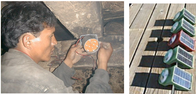
Figure ES-36. White LED Lighting System in Nepal (left) and Prototype Solar-PV Units (right)
