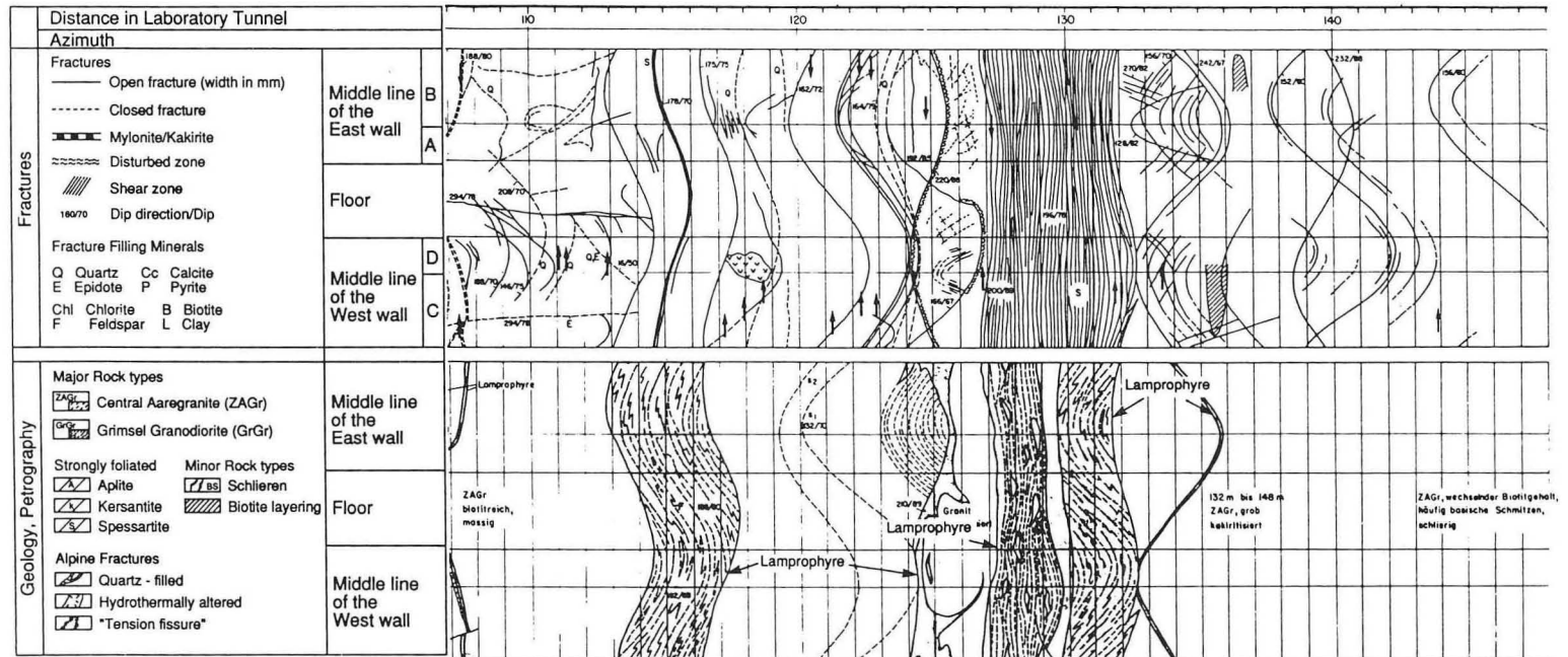
Figure 4.11a. Log of the fractures in the portion of the laboratory tunnel between L66 and L230 (from the preliminary volume of NTB 87-14).
