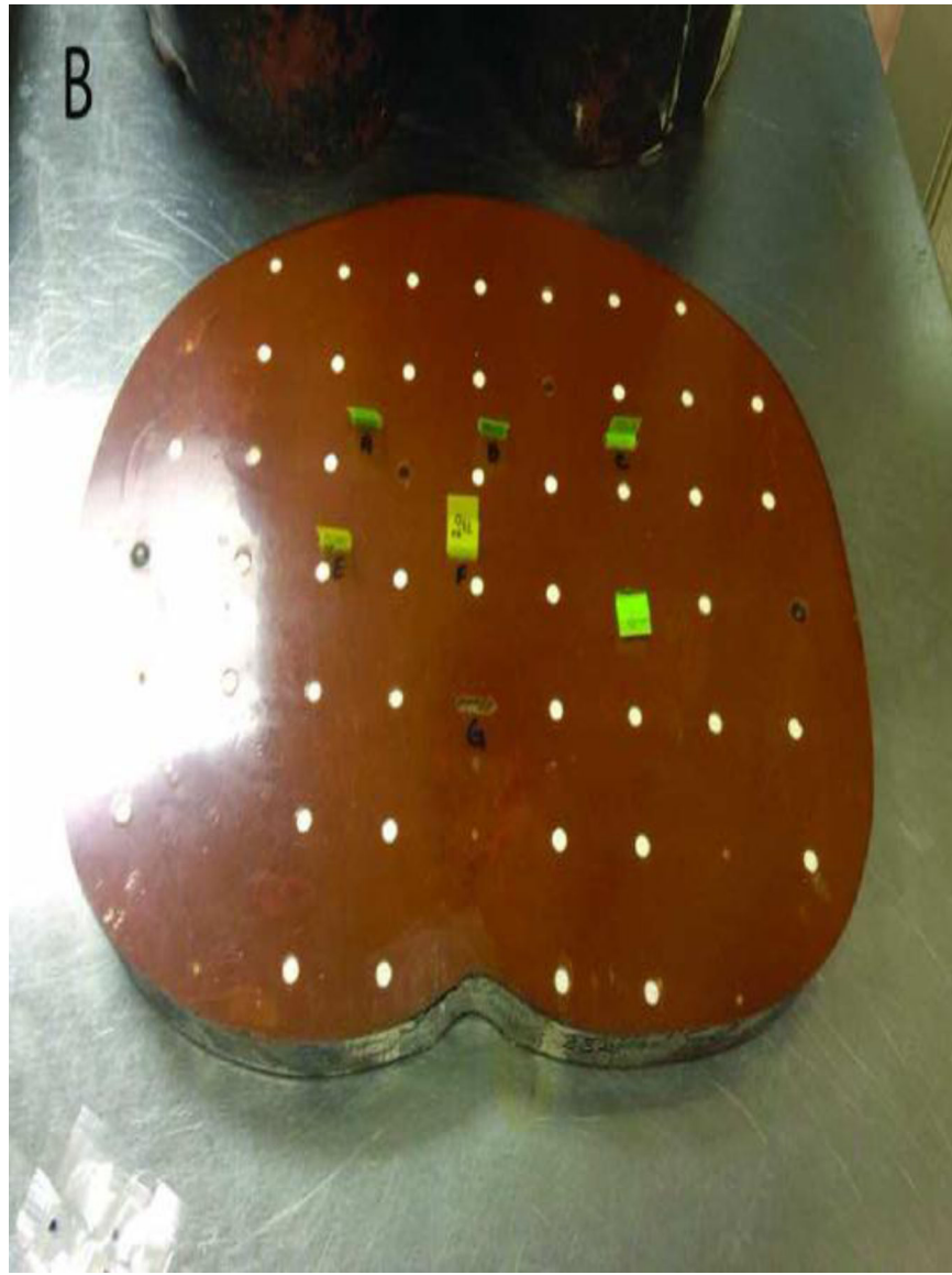
Figure 1: 1a is a picture of the anthropomorphic phantom with the cavities. 1b is a close up with the OSLDs inside the cavities.
