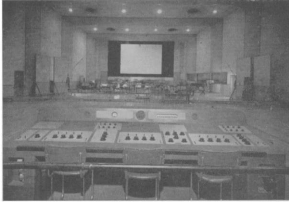
Figure 2.11: Dubbing console at Republic Studios. Image from Bloomberg, D.J., Waldon O. Watson, and Michael Rettinger. "A Combination Scoring, Rerecording, and Preview Studio." Journal of the SMPE 49 (1947), 20.
