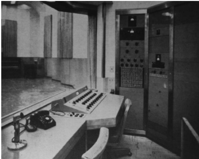
Figure 2.1: The Capitol Records Mixing Console. Image from Bayless, James W. "Innovations in Studio Design and Construction in the Capitol Tower Recording Studios." Journal of the AES 5, no. 2 (April 1957), 75.
