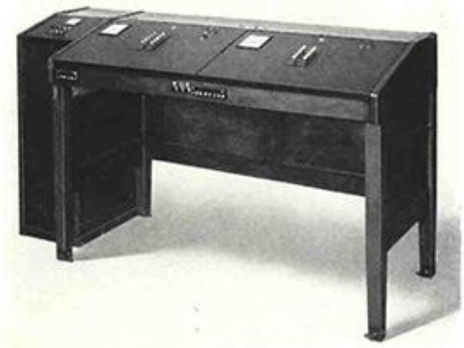
Figure 2.3: 1928 Cordless “B” Board. Image from Lacerte, W.J. “Step-By-Step Cordless ‘B’ Board.” Bell Laboratories Record 6, no. 1 (March 1928), 211.
