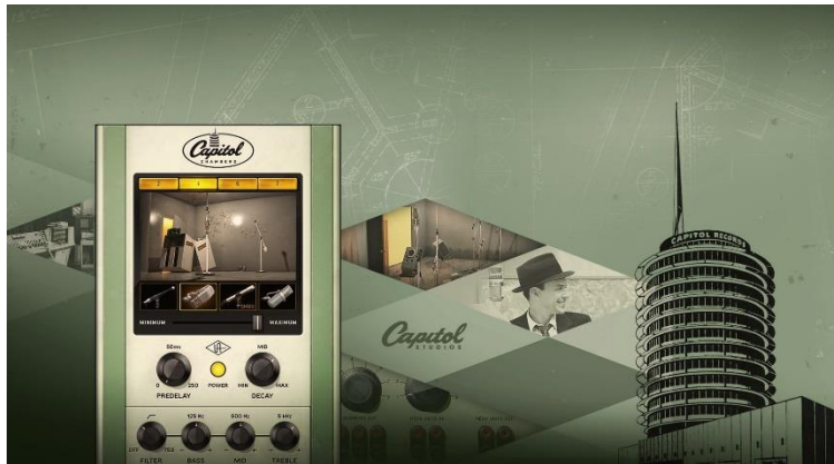
Figure 5.1: Universal Audio's "Capitol Chambers" plug-in, a digital simulation of the sonic characteristics of the reverberation chambers at the Capitol Records Tower. Image from Universal Audio website.
