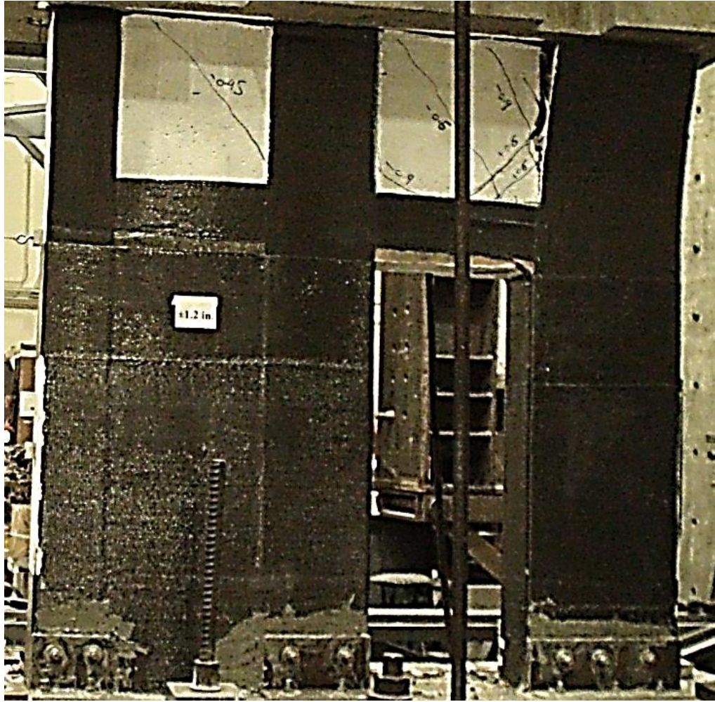
Figure (15): Failure of Wall Specimen (R-DO)
