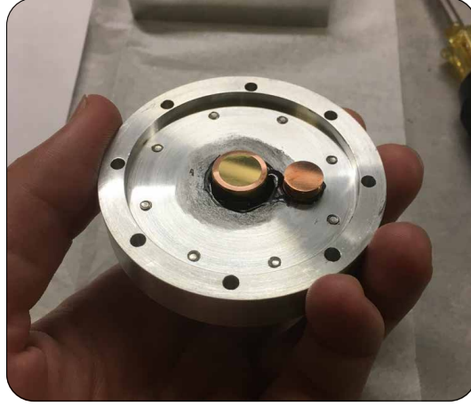
Figure 4.2: The aluminum adapter for the cavities with two electrodes. The center electrode is closer to the membrane and is typically used for the electrostatic actuation and sensing whereas the off-center electrode can be used for driving.
