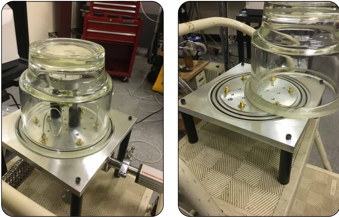
Figure 5.1: The custom vacuum chamber made to perform room temperature experiments and reduce time needed to pump down.
