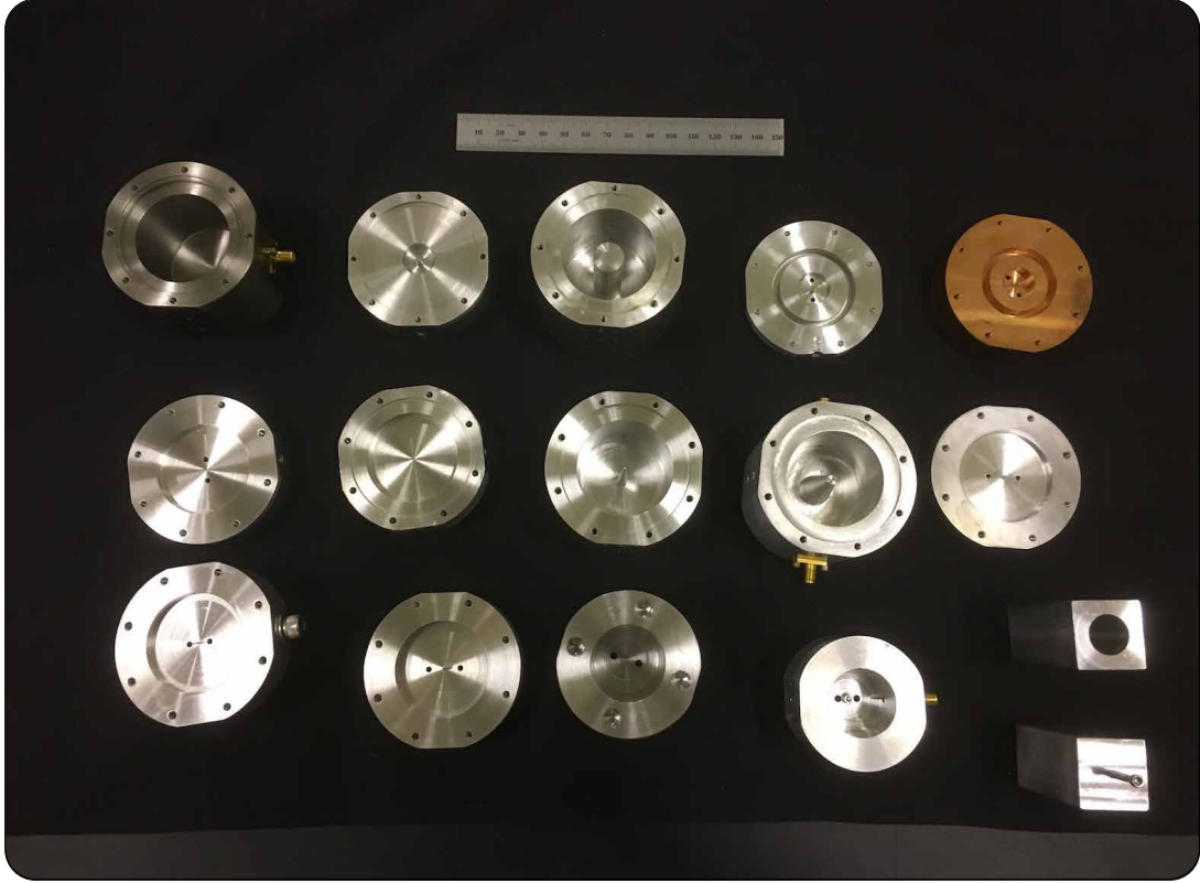
Figure 2.1: A view of the (mostly) chronological development of microwave cavities used in this thesis work.
