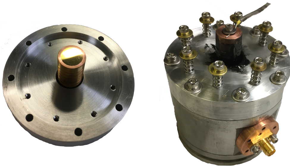
Figure 4.1: Left: The original design of the external sensing electrode adapter with aluminum bracket before bonded together. Grooves were machined into the aluminum bracket inner slot and copper electrode to have the epoxy maintain a firm grip on both surfaces. Right: The assembled design with cavity that was placed into the dilution refrigerator.
