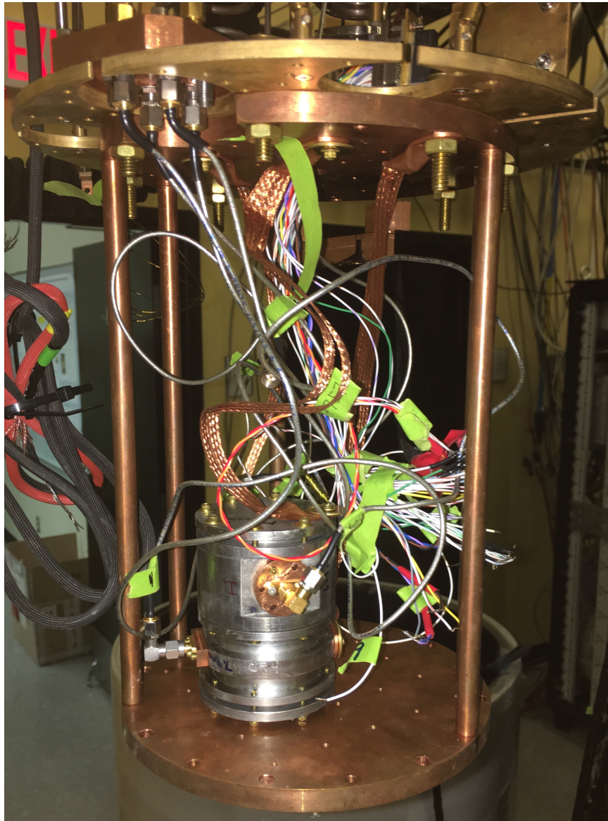
Figure 2.5: A cavity is placed at the mixing chamber plate of the dilution refrigerator. The SMA cables are connected to the cavities for transmission and reflection measurements with the amplifiers, circulators, and attenuators placed above this plate.
