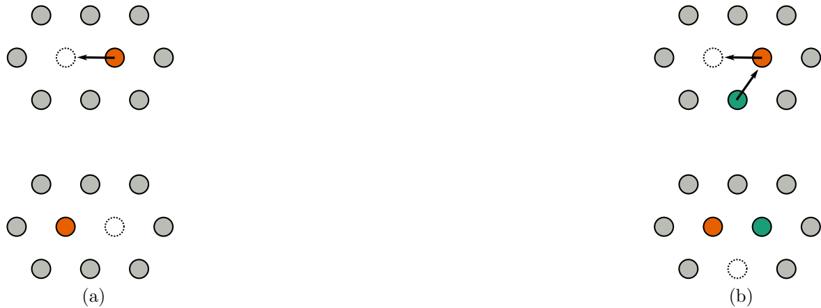
Figure 5.1: Schematic illustration of a nearest neighbor vacancy exchange (fig. 5.1a), and a cyclic hop (fig. 5.1b). Participating atoms are colored, while vacant sites are shown with a dashed circle.
