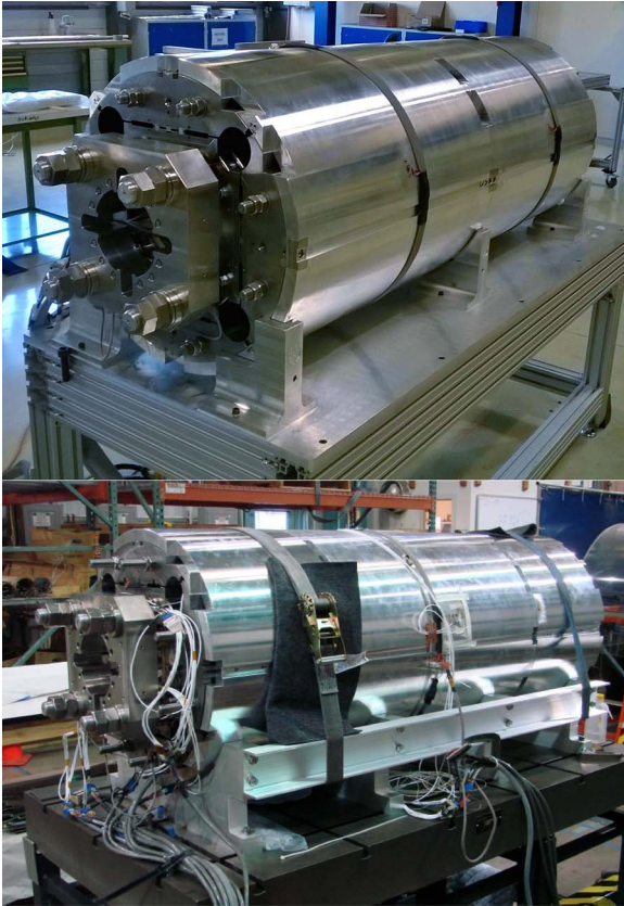
Fig. 2. (Top) MQXFSD0 structure assembled at CERN and (Bottom) MQXFSD1 structure assembled at LBNL.
