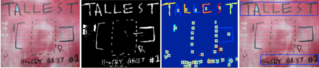
Figure 5.2: Left to right: 1. The input image. 2. Stroke Width Transform Image. 3. Connected components and geometric filtering. 4. Final Detections (blue boxes). Best viewed in color.
