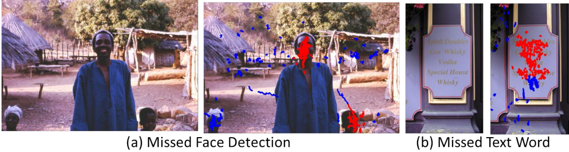
Figure 3.9: Example scenario where the proposed approach fails to detect face (left) and a text word (right). The eye tracking samples detected as face in (a) and text in (b) are shown in red and the samples detected as background (both (a) and (b)) are indicated in blue.
