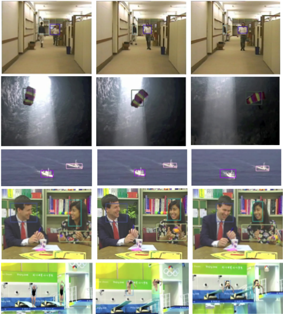
Figure 4.6: Shows example results using the proposed approach to extract multiple objects represented by bounding boxes. We see the proposed approach is able to localize different visually salient objects in the video sequences with reasonable accuracy.
