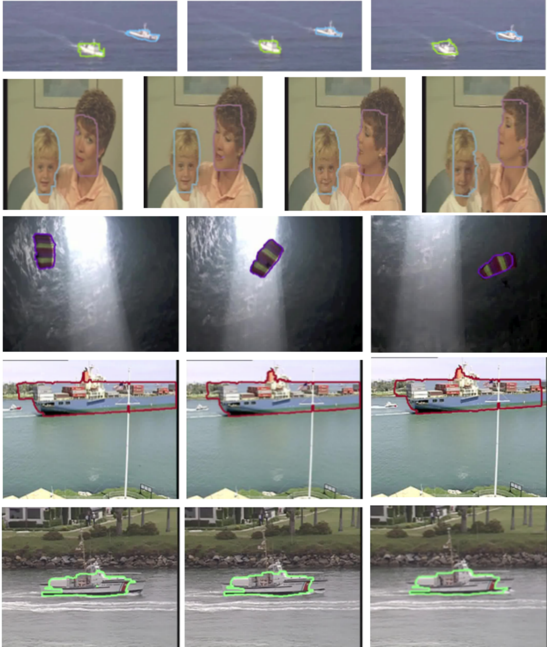
Figure 4.7: Shows example results from the proposed approach after applying grabcut based video segmentation to the extracted multiple object bounding boxes. We see the proposed approach is able to segment multiple objects in the video sequences with reasonable accuracy.
