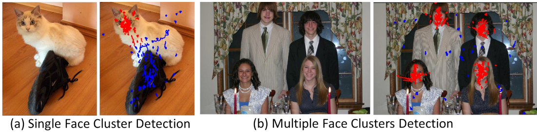
Figure 3.7: Examples of good face detections from the proposed algorithm. Red fixation points correspond to face and blue corresponds to background. (a) In the presence of salient distracting object (shoe) the face (cat) is reliably detected. (b) We notice that even in challenging scenarios where multiple faces are present, the proposed approach detects reliably.
