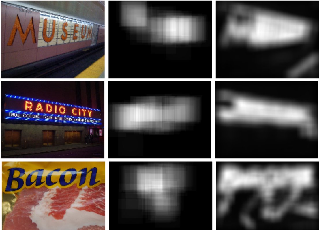
Figure 5.5: Left column shows the input image, center column corresponds to human fixation map and the right column illustrates the proposed text attention map. The text attention maps are similar to human fixation map on text centric images. Note that eye fixations only includes foveal or central vision and peripheral vision is not captured. Therefore, as row 1 and 3 only have a single word, eye tracking results are biased towards the center of the word and therefore does not entirely overlap with our text attention map. Moreover, the text attention maps reliably localize the text regions.
