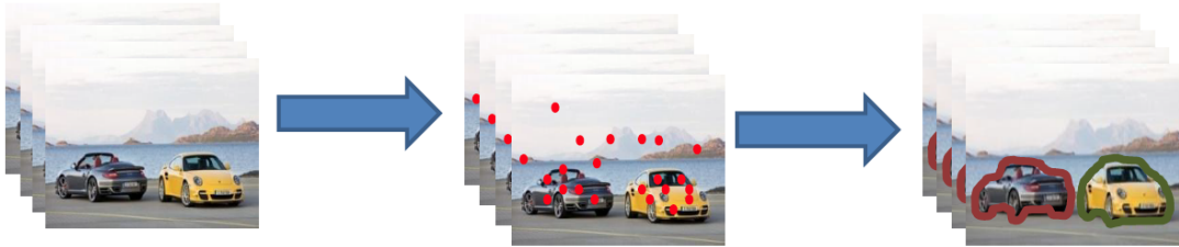
Figure 4.1: A simple illustration of the proposed problem. Given a video sequence, we collect eye tracking data in the sequence from multiple subjects and utilize this information to extract visually salient objects.
