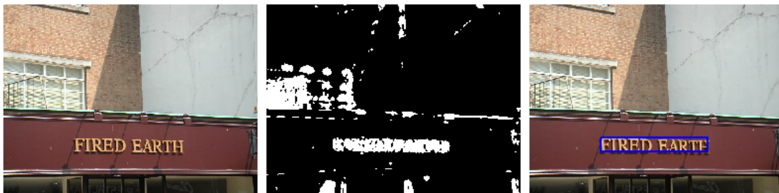
Figure 5.1: Left to right: 1. Input image. 2. Text attention map derived using visual attention features. 3. The text detection output indicated by the blue rectangle. Best viewed in color.
