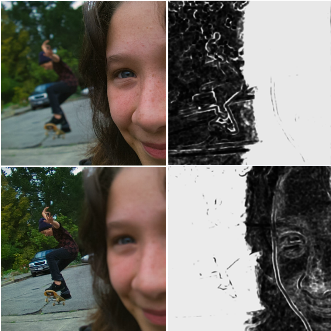
Figure 6.4: Two 2D images from a Lytro image and the corresponding binary focus maps to their right.
