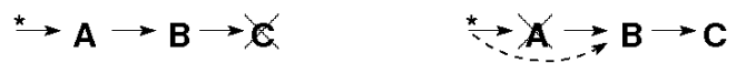
Figure 2: Left: Removal of C from a queue containing A, B and C. Right: Removal of A from a queue containing A, B, and C. Solid arrows indicate existing links, dashed arrows indicate newly created links.
