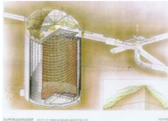
Figure 1. Cutaway view of the Super-Kamiokande detector. The detector itself stands some 42 m tall – to get a sense of the scale, consider that the tunnels shown in the drawing are large enough for full-sized trucks to drive through. The curving tunnel on the right side of the sketch contains our water purification plant; just above that is our main control room.
