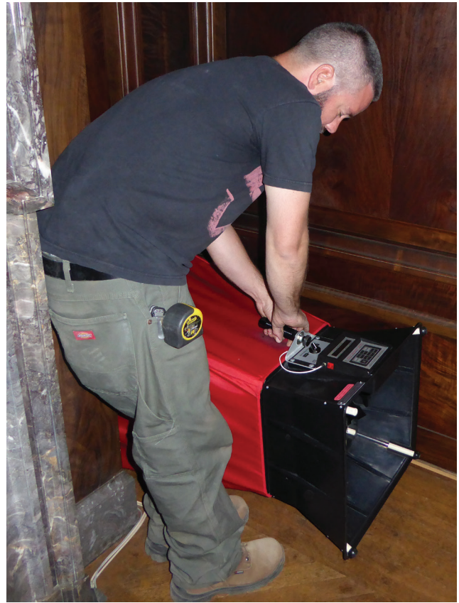
FIGURE 12 (left). Measuring discharge rates with anemometer and flow hood (right). LEFT: DAVID BITTERMANN RIGHT: MARGARET BREUKER, HACE
