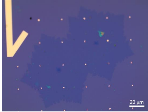
Figure S1. Optical microscopy image of a typical large area CVD graphene microcrystal. The substrate here is the standard SiO 2 /Si wafer that gives the best optical contrast.
