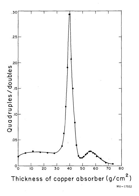
Fig. 23. Differential range curve for 102-Mev positive pion beam.
