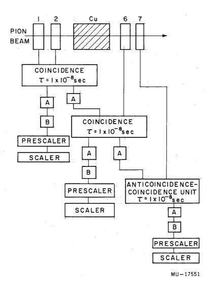
Fig. 24. Block diagram of electronics used for integral and differential range curves.
