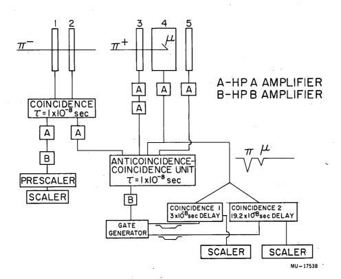
Fig. 7. Block diagram of electronics for monitor and  $\pi-\mu$  telescope.
