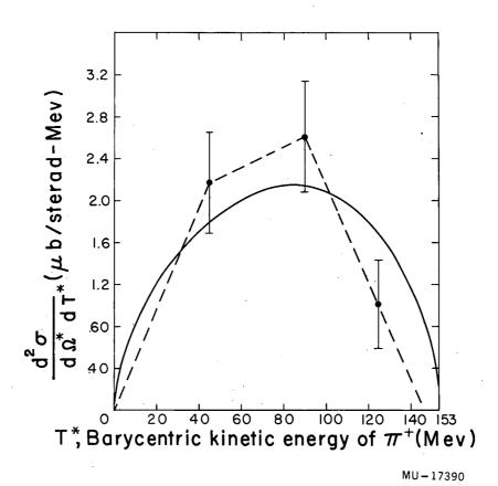
Fig. 15. Differential cross section for  $\pi^- + p \rightarrow \pi^+ + \pi^- + n$  as a function of  $\pi^+$  kinetic energy for incident  $\pi^-$  kinetic energy of 427 Mev and  $\pi^+$  barycentric angle of 90°.
