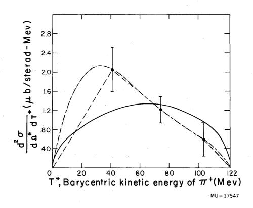
Fig. 13. Differential cross section for  $\pi^-+p\to\pi^++\pi^-+n$  as a function of  $\pi^+$  kinetic energy for incident  $\pi^-$  kinetic energy of 371 Mev and  $\pi^+$  barycentric angle of 60°.
