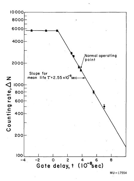
Fig. 27. Differential mean-life curve for particles counted in positive pion beam. Straight line is for  $\Delta N = \frac{N_o \Delta t}{\sigma} e^{-t/\tau}$  with  $\tau = 2.55 \times 10^{-8}$  sec.
