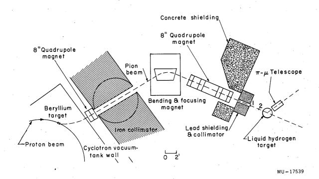
Fig. 1. Diagram of experimental arrangement.
