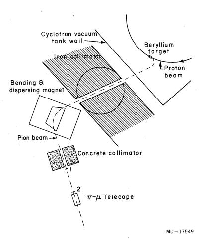
Fig. 21. Experimental arrangement for calibration of  $\pi$ - $\mu$  telescope with positive pion beam.
