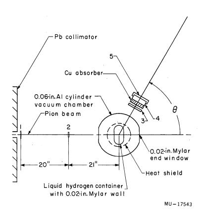
Fig. 6. Diagram showing details of hydrogen target and counter arrangement.
