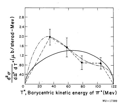
Fig. 14. Differential cross section for  $\pi^- + p \rightarrow \pi^+ + \pi^- + n$  as a function of  $\pi^+$  kinetic energy for incident  $\pi^-$  kinetic energy of 371 Mev and  $\pi^+$  barycentric angle of 90°.
