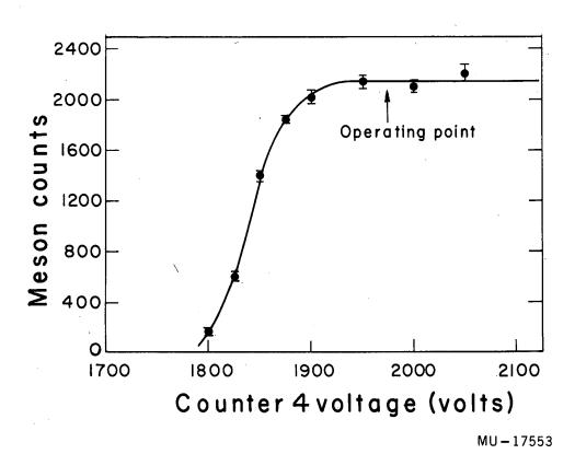
Fig. 25. High-voltage plateau curve of Counter 4.
