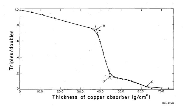
Fig. 22. Integral range curve for 102-Mev positive pion beam.
