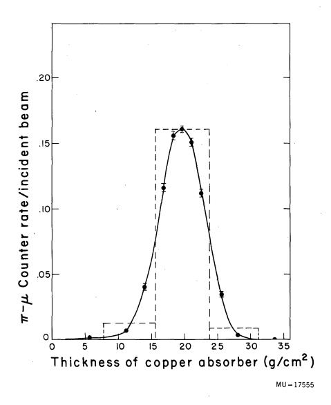
Fig. 28. Calibration curve for  $\pi$ - $\mu$  counter telescope.
