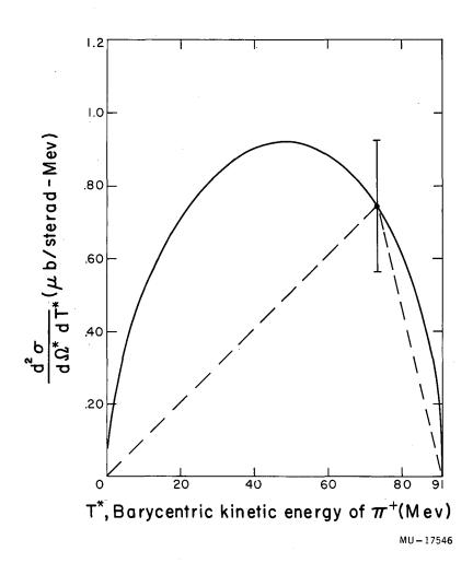
Fig. 12. Differential cross section for  $\pi^- + p \rightarrow \pi^+ + \pi^- + n$  as a function of  $\pi^+$  kinetic energy for incident  $\pi^-$  kinetic energy of 317 Mev and  $\pi^+$  barycentric angle of 1590.
