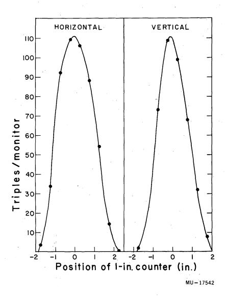
Fig. 5. Horizontal and vertical beam profiles taken with a l-in.-diameter counter at the position of the liquid hydrogen target.
