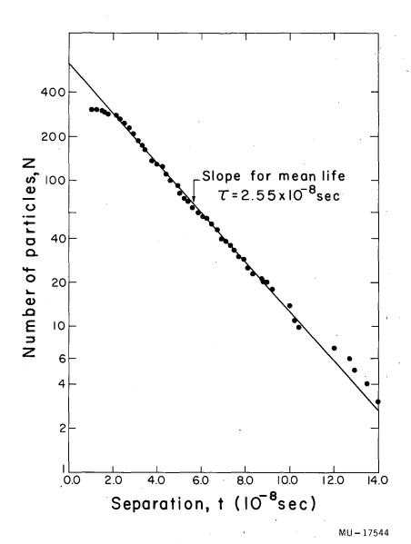
Fig. 8. Integral mean-life curve for particles produced by 371-Mev negative pions in liquid hydrogen target. Straight line is for  $N = N_0 e^{-t/\tau}$  with  $\tau = 2.55 \times 10^{-8}$  sec.
