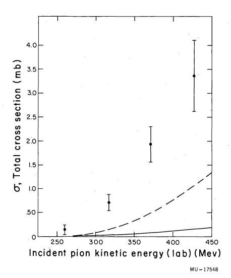
Fig. 19. Total cross section for  $\pi^- + p \rightarrow \pi^+ + \pi^- + n$  as a function of the  $\pi^-$  kinetic energy (lab). The curves are the theoretical predictions based on the static model. The solid curve is prediction by Kazes 16 while the dashed curve is the prediction by Franklin. 14
