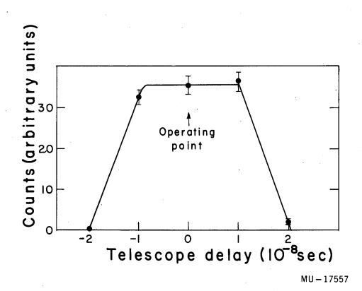
Fig. 26. Delay curve between monitor counters and  $\pi$ - $\mu$  counter telescope.
