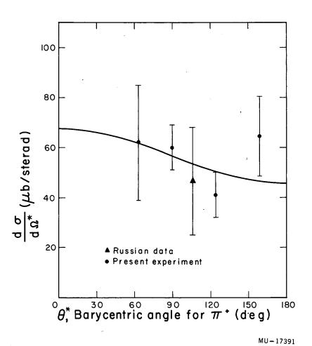
Fig. 16. Angular differential cross section for  $\pi^+$  meson for an incident  $\pi^-$  meson of 317 Mev.
