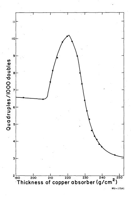
Fig. 4. Differential range curve for 371-Mev negative pion beam.
