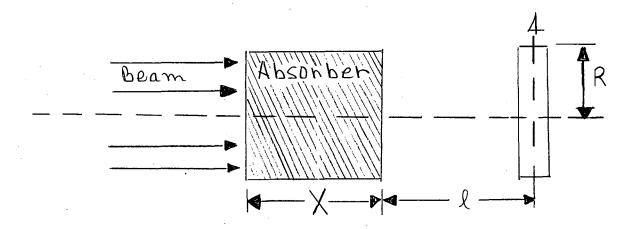
For a parallel, uniform beam of radius  $\rho_{o}$  passing through an absorber of thickness x at a distance  $\ell$  from a counter of radius R, the fraction of the beam that strikes the counter is F (r\_{o}^{!}, \rho\_{o}^{!}). F is a function of only  $\rho_{o}^{!} = \rho_{o}/R$  and the quantity
