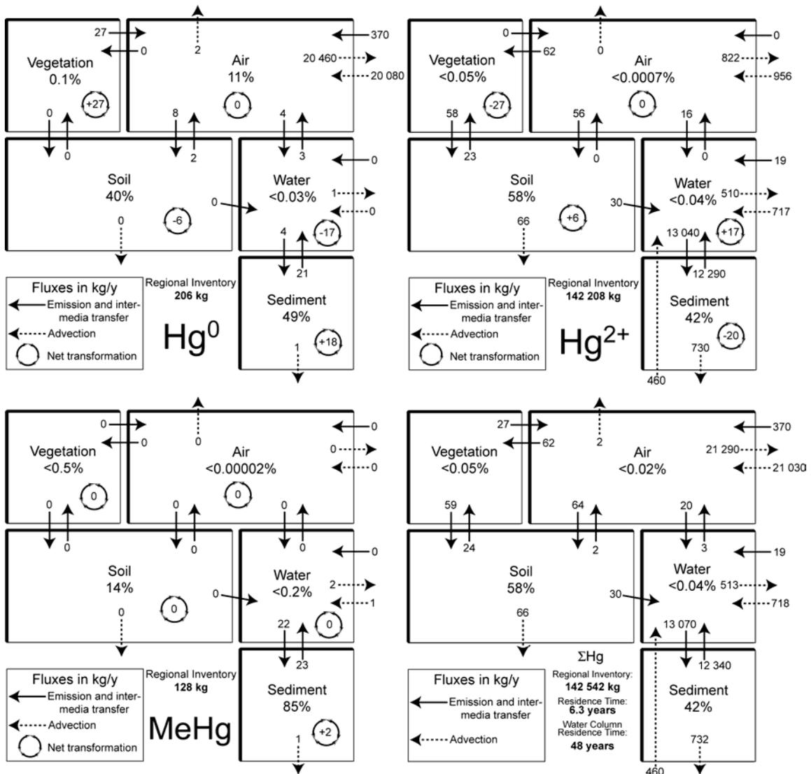
Figure 5. Steady-state mass balance of elemental mercury ( $Hg^0$ ), divalent mercury species ( $Hg^{2+}$ ), methylmercury species (MeHg) and total mercury ( $\Sigma Hg$ ) in the San Francisco Bay Area. Fluxes are rounded to the nearest 1 kg/y or 4 significant digits. Percentages are of the total quantity of each mercury species.
