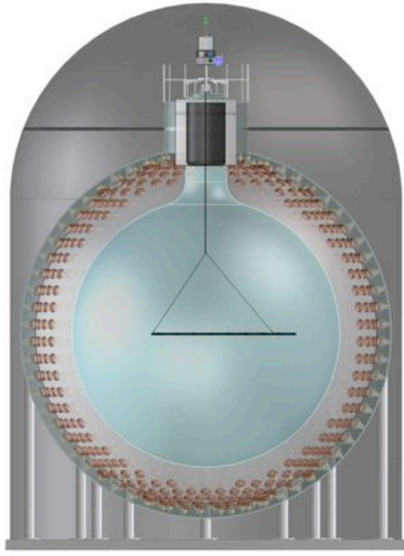
Figure 1. Illustration of the calibration system in the KamLAND detector: A radioactive source was attached to one end of the pole. It was positioned throughout the fiducial volume by adjusting the orientation and length of the pole. Additional ^{60}\text{Co} pin sources, used for monitoring the pole position, were located along the pole. Two cables and a spool system manipulated the pole position and provided electrical connections to instrumentation in the pole. Access to the detector and manipulation of the system was through a glovebox on top of the chimney.
