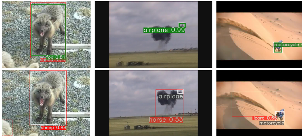
Figure 4.4: Naturally perturbed examples for detection. Red boxes indicate false positives; green boxes indicate true positives; white boxes are ground truth. Classification errors are common failures, such as the fox on the left, which is classified correctly in the anchor frame, and misclassified as a sheep in a nearby frame. However, detection models also have localization errors, where the object of interest is not correctly localized in addition to being misclassified, such as the airplane (middle) and the motorcycle (right). All visualizations show predictions with confidence greater than 0.5.
