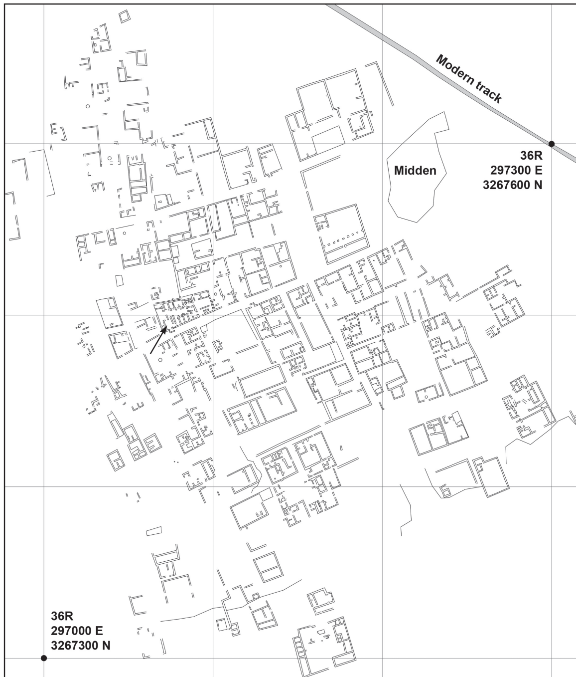
FIG. 9. Measured plan of Karanis East prepared in 2008 by Hans Barnard, Erwin Bolhuis and Sander Tiebackx (University of Groningen) using a Topcon GTS-235W total station. All coordinates are projected onto Zone 36R of the WGS84 geode. North is at the top of the map, each box is 100 by 100 m square. The arrow indicates the position and direction in which the photograph in figure 10 was taken; 36R—297000 E—3267300 N at the bottom left equals 29°N 31'07.8"—30°E 54'19.8".
